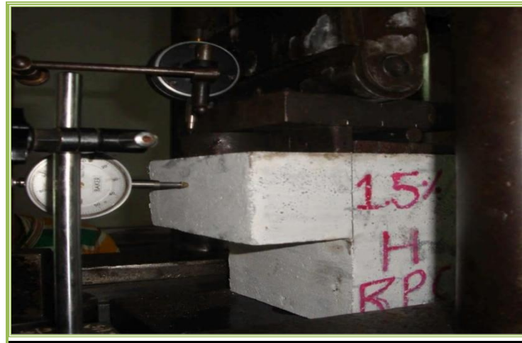
FIG 4.0: PHOTOGRAPH OF EXPERIMENTAL SET-UP FOR SHEAR STRENGTH TEST
